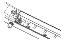
Insert the Lower support bracket into the bottom part of the frame and with 2 M5\*10 screw fix it into position.
