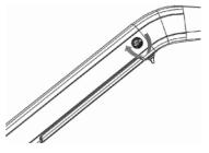
2. Then using the lever, push the lever up to release the second locking mechanism.
