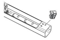
4. Place cable cover into the frame ensuring all cables are in the correct position and not crossing each other. Now using 3 x M5\*6 mm screws tighten the cable cover into position.
