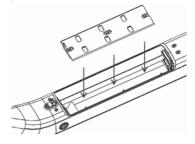
Place the Battery Cover on top of the battery ensuring each corner sits comfortable into the groves provide on the battery.
