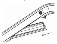
8. Now push the top part of the battery into the frame, until you hear the battery lock into position, and the battery cover sits flush with the frame.
