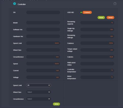
Please read first then write Wheel Size, Circumference and Speed Limit. If the read speed Limit is 25km/h, then the maximum speed limit is 25km/h. If the read speed limit is above 25km/h, the maximum is what read from HMI.
