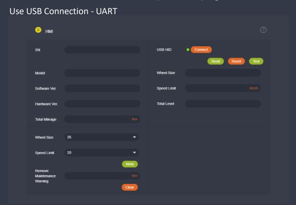
Please read first then write Wheel Size and Speed Limit. If the read value of speed Limit is 25km/h, then the maximum speed limit is 25km/h. If the read value of speed limit is above 25km/h, the maximum is what read from HMI.
