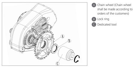
Put the chain wheel onto the spline shaft of the drive unit. Use a dedicated tool to fasten the lock ring onto the spline shaft. Torque: 35 Nm.
