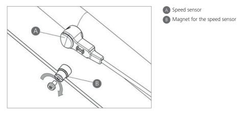
Fasten the mounting screws through the speed sensor and with a cross screwdriver. Tightening the speed sensor onto the frame. Then place the rubber seal on the speed sensor hiding the screw. Torque requirement: 1.5-2 N.m.
