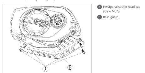
As shown in the figure, use internal hexagonal wrench to tighten 2 M5\*8 screws through hole sites on the bash guard to the connection interface(right side as shown in the figure), with tightening torque at 4 N.m. Then, use internal hexagonal wrench to tighten 2 M5\*8 screws through hole sites on the connection interface to the bash guard(left side as shown in the figure), with tightening torque at 4 N.m.
