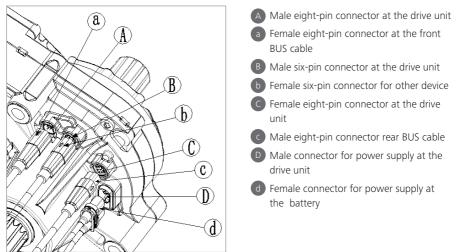
First link the female connector (8 pin) from EB-BUS a to the male connector (8 pin) at the drive unit A. Then link the male connector (8 pin) from EB-BUS c to the female connector (8 pin) at the drive unit C, finally link the power connector together. (Link 6 pin EB-BUS to drive unit this is based on customer functional requirements)
